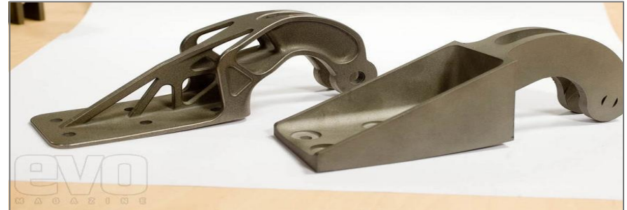
Optimized A320 Nacelle Hinge – DMLS and Conventional EOS Ti64 produced on EOSINT M 270Xt at EADS IW
